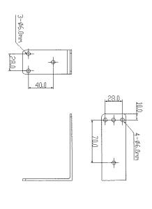
Stpe1: 3 holes on the wall then 3 expansion screws into the hole, as arrow points
